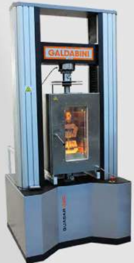
Universal testing machine Quasar 200 with Micron Motor MFX extensometer and thermostatic chamber
